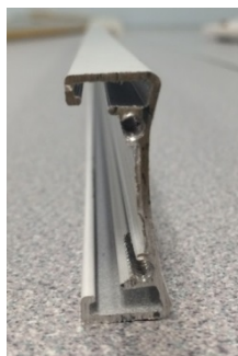
When aligning the bracket with the headrail for attachment, make sure the screws flow through the holes in the bracket directly into the small grooves in the headrail.
