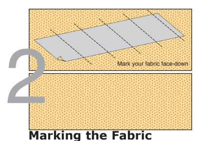
Position the finished shade fabric "face down" on your work table. The various pleat positions should be marked on the fabric. Make sure the bars will be parallel to each other and are 90° to the fabric edges. Once marked, flip the fabric over so it it is now "face-up" onto the table.
