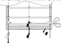
**NOTE:** The cord tension may be adjusted by pulling the plug out of the bottom pocket and sliding the plug up or down until the tension is correct. When tension is equal on all lift lines, insert the plugs back into the bottom pockets.
