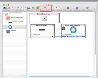
Make a connection between the "RS232 to RS485 Adapter" port on Shade Controller profile and the RS232 port on the Savant Extender. Please keep in mind, Savant currently only supports RS232 control for this device, so an RS485 adapter is needed. Then click the "Generate Services" button.
