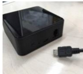
3. Insert the micro USB end of the power cord (long or short) into the Wi-Fi bridge.
