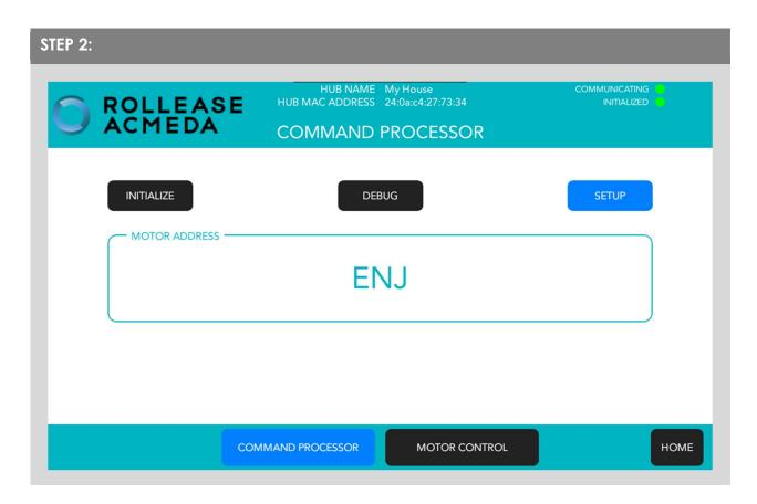
11. Once you have the address for all your desired motors, uncomment the "MOTORADD" commands in the example program (lines 118 – 122) and enter in the appropriate address in the command for each motor (the example program has 5 motors. You may have more or less in your installation). Once the addresses have been entered, recompile and reload your program.).
