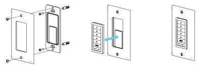
Use supplied fasteners and anchors as needed to attach the base and cover.
