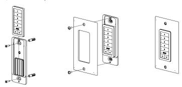
Slide the Switch onto the Wall Clip.
