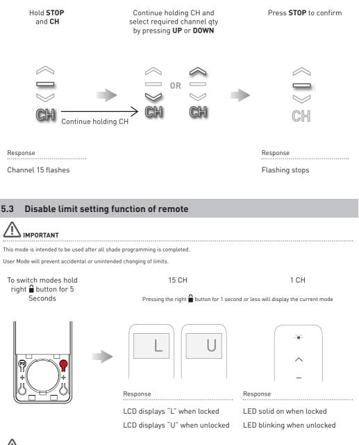
It is still possible to add or delete channels and perform **P2** functions, while the lock function is enabled.
