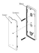
Replace cover by pressing snap latches into place.
