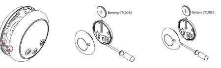
Replace cover by aligning notches and press together.
