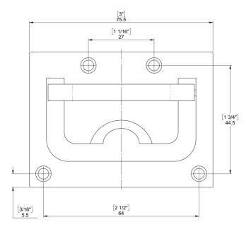
Note: Countersunk #6 fasteners required. Not supplied.
