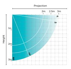
Wall Mounting: 3° to 70° Roof Mounting: 11° to 90° Depending on manual or crank.
