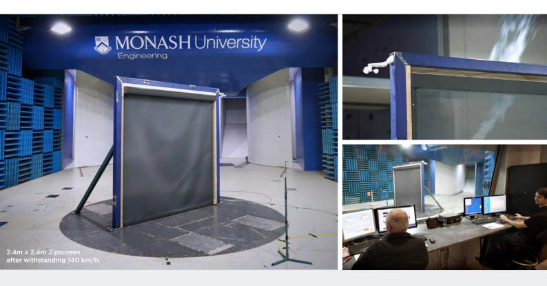
\*The Zipscreen shade was side fixed to a timber substrate and secured to a steel frame with 12G fasteners. Inner rails were secured with 8G fasteners as per the Zipscreen Installation Manual guidelines. Each wind speed test was held for a minimum of 60 seconds. 'Maximum achievable wind speed' refers to the limitations of the testing facility, and not the Zipscreen system.
