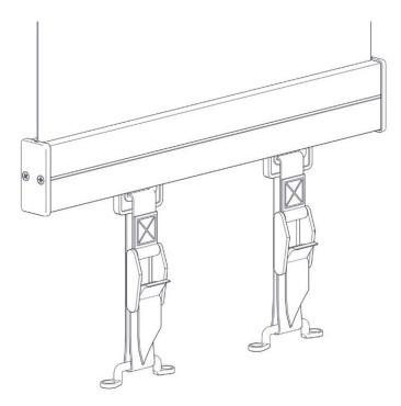
NOTE: Ensure straps are adjusted so that the weight bar is level.
