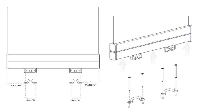
STEP 2 - ATTACH CLIP IN CORRECT ORIENTATION
