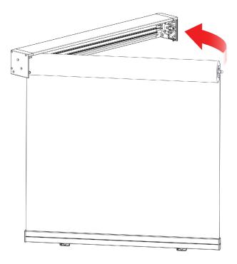
User effort will be required to push the booster head/Idler pin into the adapter, a noticeable "click" will indicate that the component is correctly located.
