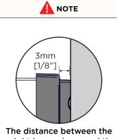
weight bar end cap and the edge of the inner rail should always be approximately 3mm [1/8"].
