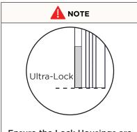
Ensure the Lock Housings are perfectly level. Test this by lowering the weight bar into the Ultra-Lock housings (both pins should click at the same time). Adjust position of Inner Rails as required.
