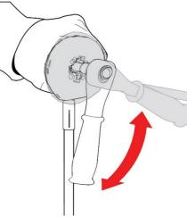
To re-lock the booster and shade, while holding the shade, release the wand control and rotate the Socket Ratchet enough to re-engage the lock (approx. ¼ turn). The ratchet should move back under the booster tension to the locked position.
