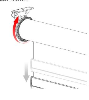
To raise the top limit position rotate limiter head so that the Shade raises.
