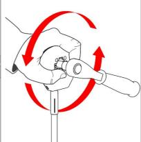
While holding the shade, grip the wand control head and also prevent both from turning. To add tension, rotate the Socket Ratchet for the number of turns desired in a counter clockwise. (Note, to remove tension allow the spring to unwind in the clockwise direction)
