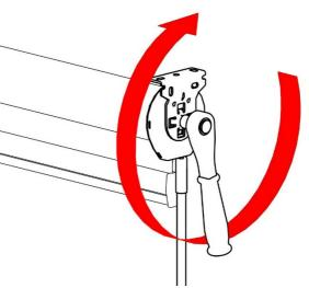
NOTE: If there is insufficient space to rotate Socket Ratchet within installation, Shade will need to be removed from the bracket to undertake process.
