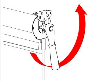
NOTE: If there is insufficient space to rotate Socket Ratchet within installation, Shade will need to be removed from the bracket to undertake process.
