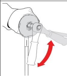
Hold the shade and use the Socket Ratchet to rotate the adjusting shaft (and wand control head) in an anti-clock wise direction enough to release the booster lock. The ratchet will move back under the spring tension.
