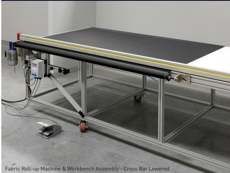
Fabric Roll-up Machine & Workbench Assembly - Cross Bar Lowered
