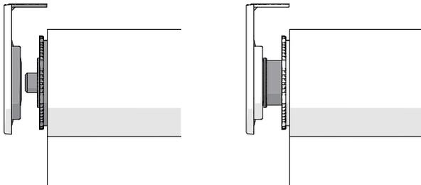
Rotate disk clockwise to extend the pin in 1mm increments.
